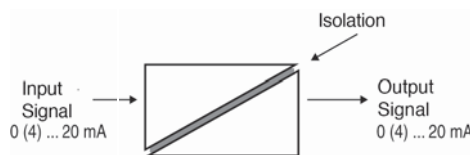
Figure: Passive isolation, supply input
